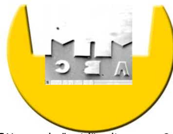
TEM sample "grid", diameter 3mm
